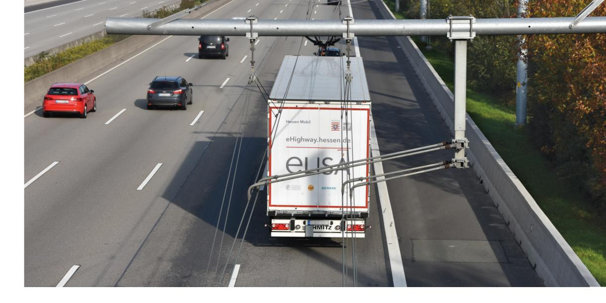
n the second phase of the ELISA project, the eHighway system will be tested over a period of four years until the end of 2022, both on the vehicle and infrastructure side.
